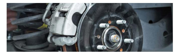
Brake pads fall under the consumable category when it comes to car parts. They wear down over time and eventually need replacing. Because of this, it's important to keep an eye on the amount of brake pad material that remains on the brake pads, keeping both your customer and their family safe on the roads.
