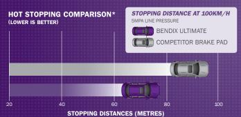
\*"HOT" STOPPING DISTANCE CALCULATED AFTER TEN CONSECUTIVE 0.5G DECELERATION STOPS FROM 100KM/H DURING B8E4-55 DYNAMOMETER STANDARD PERFORMANCE TEST.
