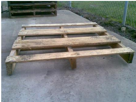
X Missing planks
