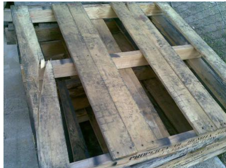
X Cracked planks
