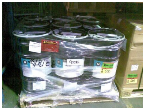
✓ Stabilised load well labelled
