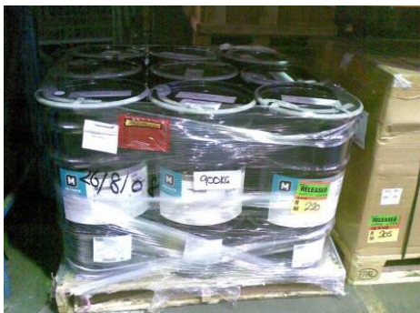
✓ Stabilised load well labelled
