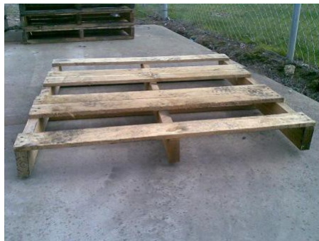
X Missing planks
